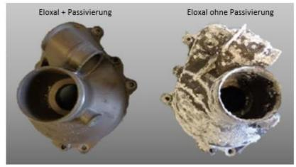
Application on anodized surface - here AI - casting material (layer thickness 3-10  $\mu m$ ). No corrosion after 720h neutral salt spray test according to EN ISO 9227 NS
